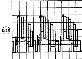
IC301 pin ⑦ (EE) 20μs/div. 200mV/div.
